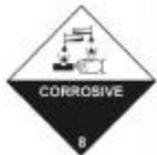
**IMDG / IMO****UN no:** 1759**Class:** 8**Packing group:** III**EmS:** F-A,S-B**Marine pollutant:** .**Labelling:** 8**IATA / ICAO****UN no:** 1759**Class:** 8**Packing group:** III**Packing instructions:** 822(P&CA); 823(CAO)**Labelling:** 8
